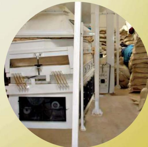
Gravity Separator Section
